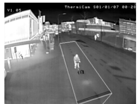
Thermal cameras do not rely on visible light and can, therefore, detect bicyclists and vehicles 24/7 and in adverse weather conditions.
